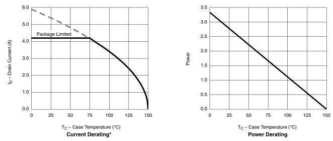
\* The power dissipation  $P_D$  is based on  $T_{J(max)} = 150 \text{ °C}$ , using junction-to-case thermal resistance, and is more useful in settling the upper dissipation limit for cases where additional heatsinking is used. It is used to determine the current rating, when this rating falls below the package limit.
